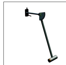
Pendulum impact hammer with angle scala
